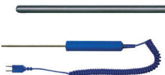
Sonde air/liquide X13 Ø 3 mm x L = 130 mm 1/2 DIN 1000 °C max.
